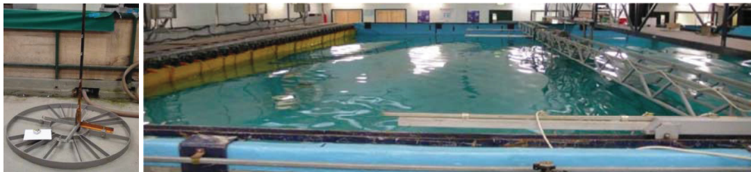
Figure 1. Photographs of ocean wave testing basin and model monopile.
