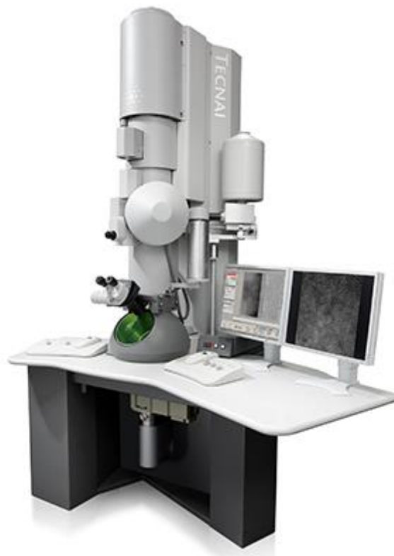
Fig. 3.7. TEM instrument for micro structural analysis of materials
