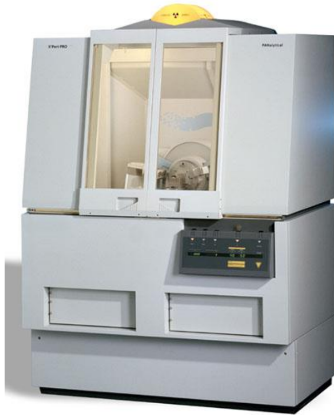
Fig. 3.12. Image of PANalytical X'Pert Pro MPD X-ray Diffractometer (XRD) used for structural characterization of the materials.
