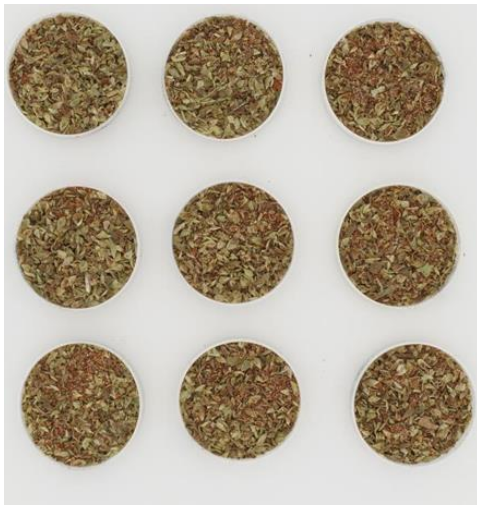
Figure 7.5- Progression of mixing for the 9 samples at 2 and 30 seconds for a) for oregano-salt and b) poor mix
