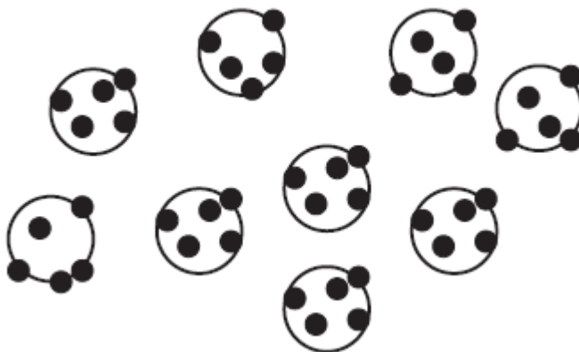
Figure 2.2- Fine particles adhered to carrier particles (Barbosa-Cánovas et al., 2005b)
