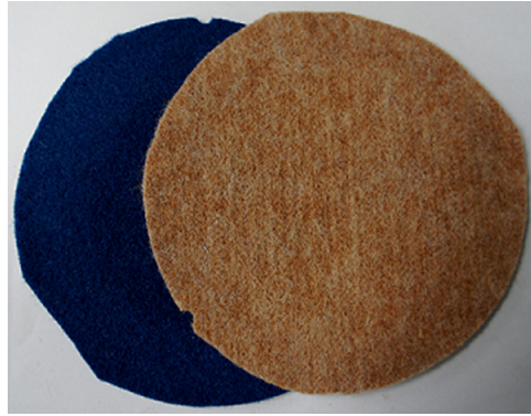
FIG. 4. Porous damping disk for representing linear air flow damping.
