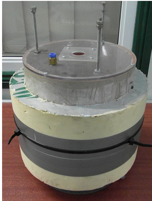
FIG. 1. A generic cylinder OWC wave energy converter.
