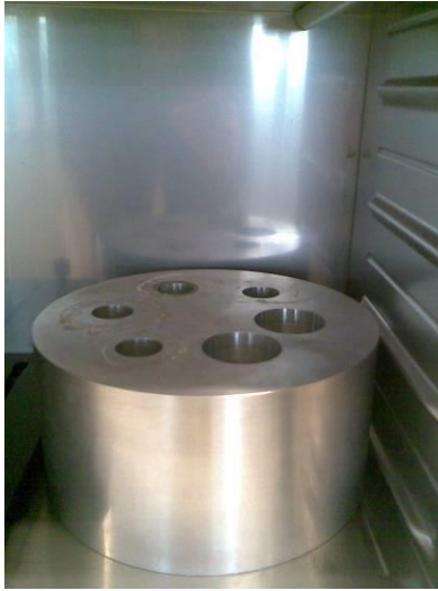
Figure 2.5 A photograph of the aluminium block used to stabilise sample temperature during controlled evaporation
