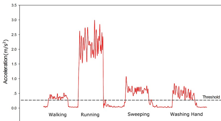
Figure 5.5: Standard Deviation threshold for trunk accelerometer signals
