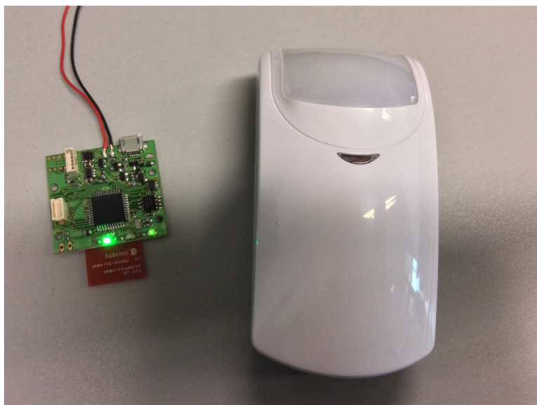
Figure 4.4: Prototype of the PIR sensor
