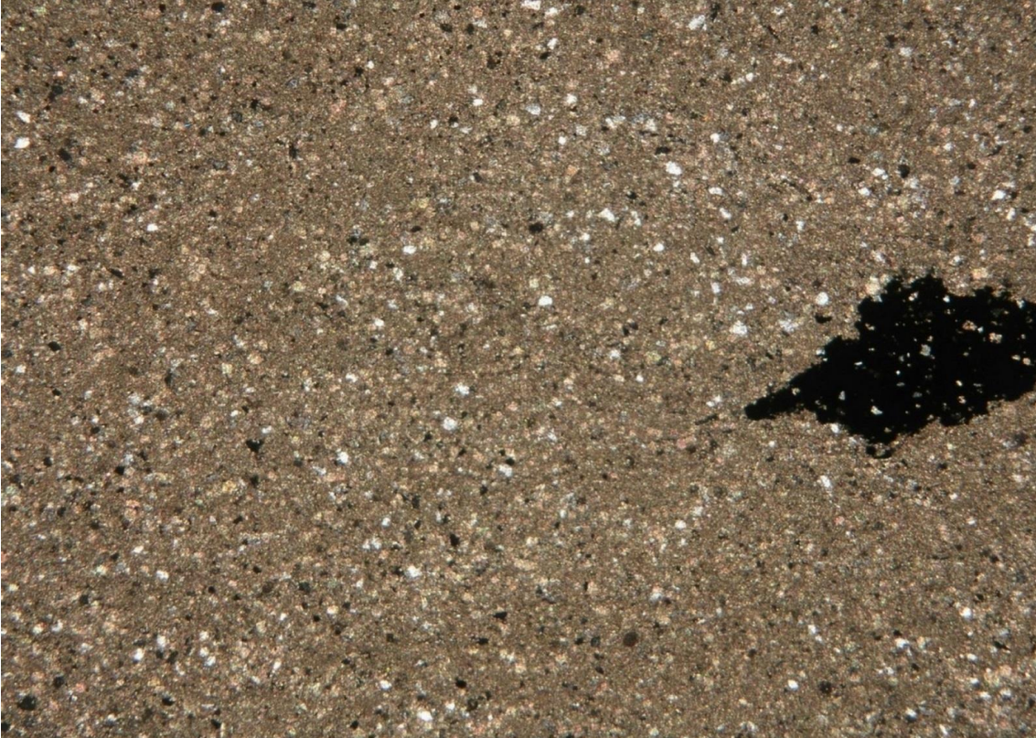
Figure 4. 221 Thin section of sample Wy3. Field of view is approximately 4mm. The fine grained texture observed is typical of the Allan Mountain Limestones studied and is too fine grained for accurate strain analysis
