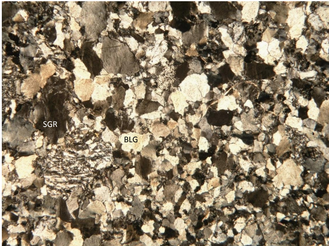
Figure 6. 30 Microstructures observed in the Crows Point Formation from Whiting Bay. Grain boundary bulging (BLG) and sub grain rotation (SGR) appear to be the dominant deformation mechanisms. Image is approximately 2mm across.
