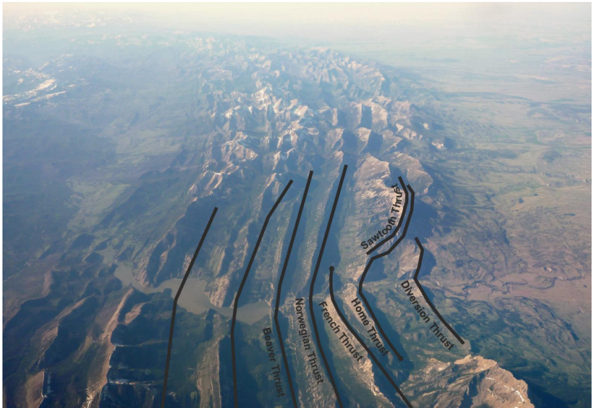
Figure 4. 2 Aerial photograph looking north across the Sawtooth Range, the Gibson Reservoir is right foreground and the Sun River extends eastward from the reservoir. Thrust geometries can be clearly seen with consistent westward dips.
