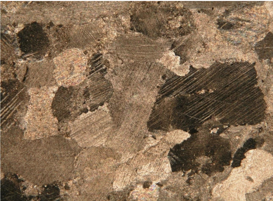
Figure 4. 212 Thin section of sample Wy18. Field of view is approximately 4mm. The coarse grained texture while ideal for strain analysis is rarely observed. Microstructural deformation observed is mainly grain boundary bulging and calcite twinning.
