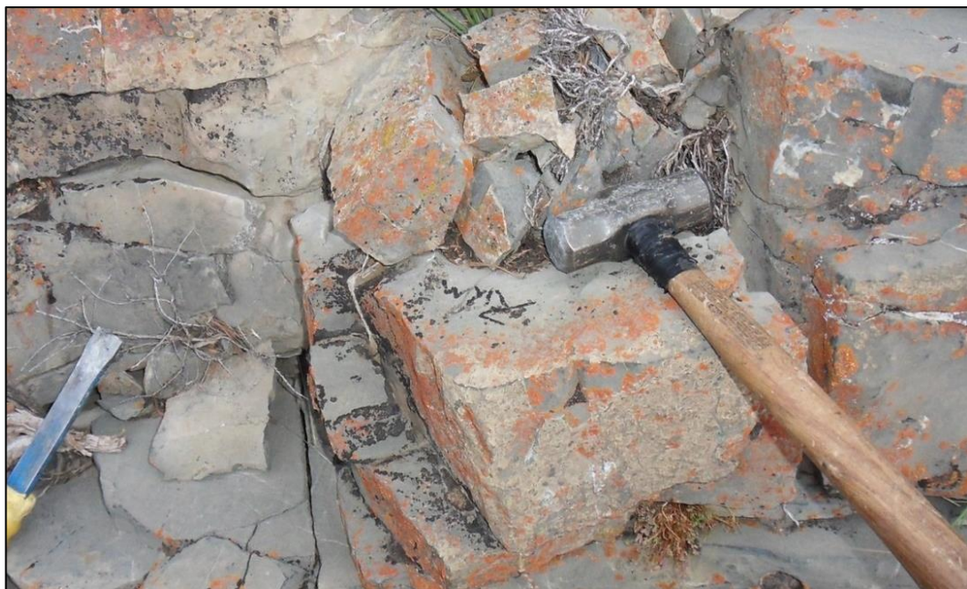
Figure 3. 13 Block marking prior to extraction.
