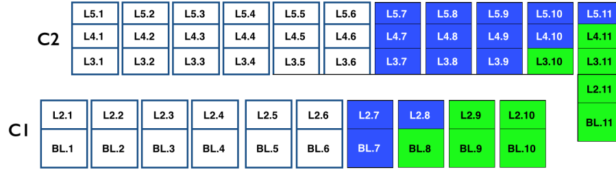
Figure 5.7: Two streaming classes created from ALD with five-layer and an STF of 6. C1 denotes class one and C2 denotes class two
