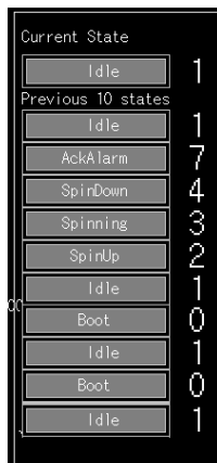
Figure 10 HMI screen shot of state log
