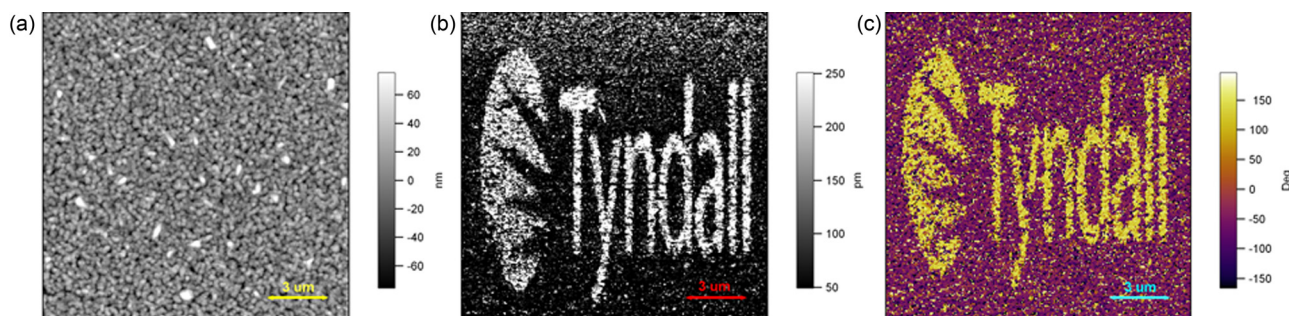
FIG. 11. Images of BTF7M30 on SiO 2 -Si: (a) topography, (b) out-of-plane PFM amplitude, and (c) out-of-plane PFM phase after PFM lithography with an applied dc bias of 33.0 V.
