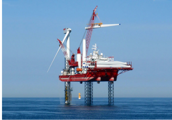
Figure 1-7: Wind turbine installation vessel at the Sheringham Shoal wind farm [6]
