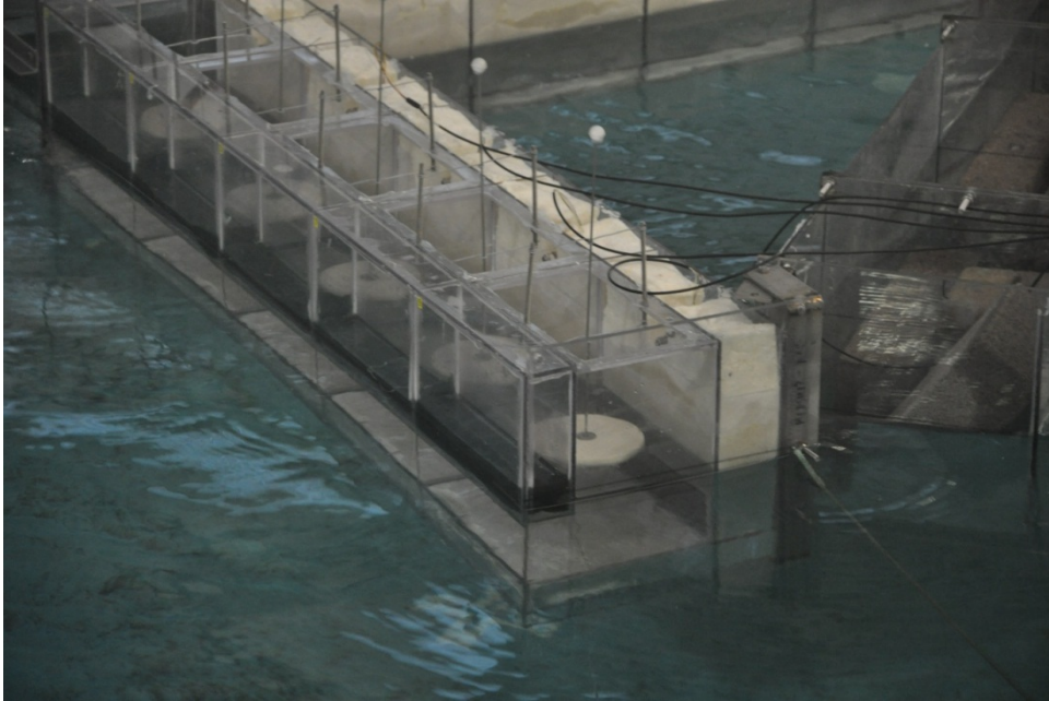
Figure D.7: Float, guides and Qualysis maker arrangement in the chamber
