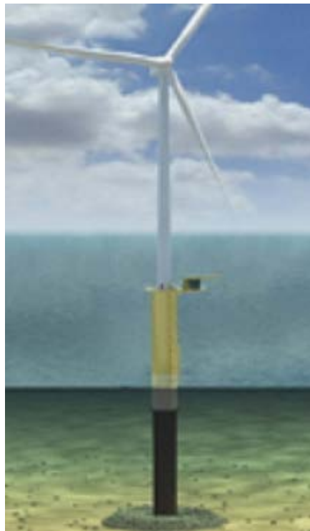
Figure 2-46: A typical monopile foundation
