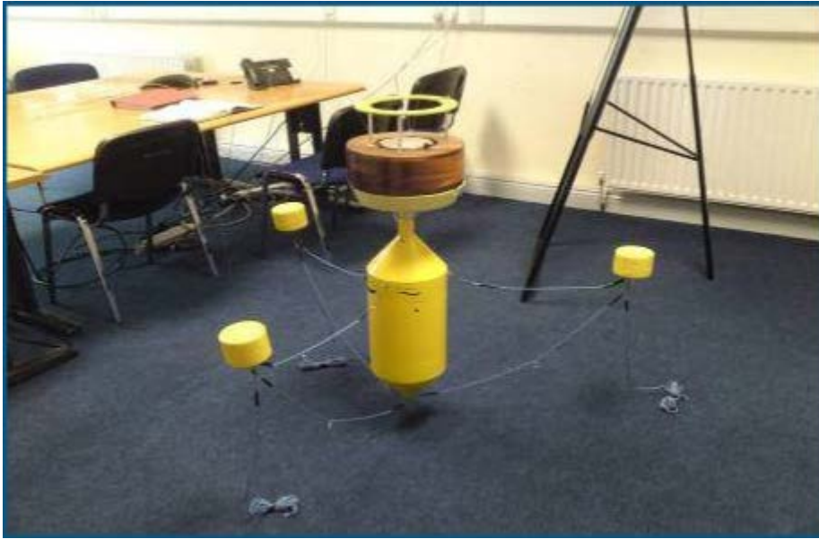
Figure 2-22: Wavebob Conceptual Mooring System
