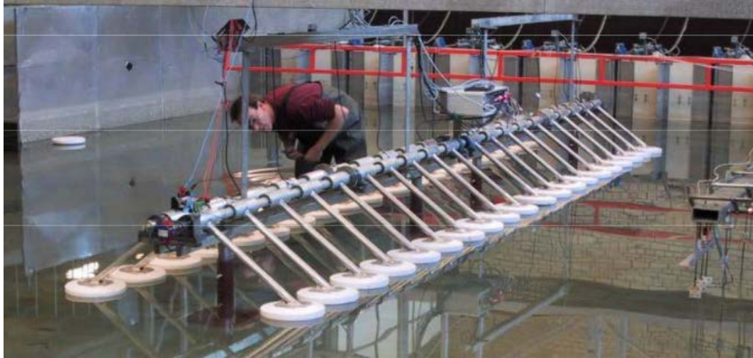
Figure 2-26: Wavestar 1:40 Model at Aalborg University
