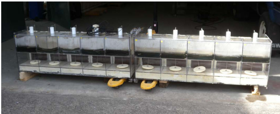
Figure D.11: Full chamber beam in dry test simply supported
