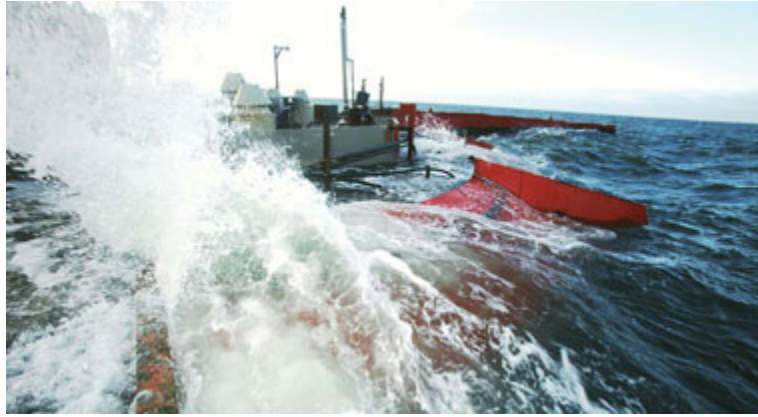
Figure 2-42: 1:4.5 Scale Model of Wave Dragon at Nissum Bredning
