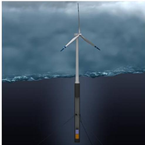
Figure 2-53: The Spar Floating Wind Turbine and Delta Mooring Line Concept ([76], [77])
