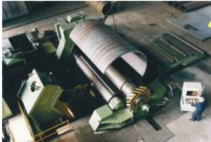
Figure 3-13: Monopile “Can” Rolling
