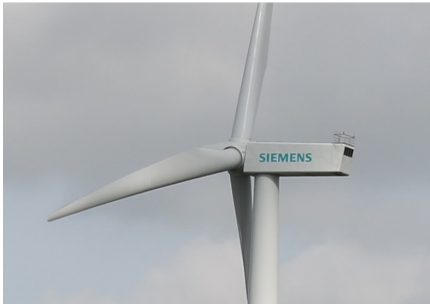
Figure 2-44: The Siemens SWT-3.6-120 3.6MW Turbine
