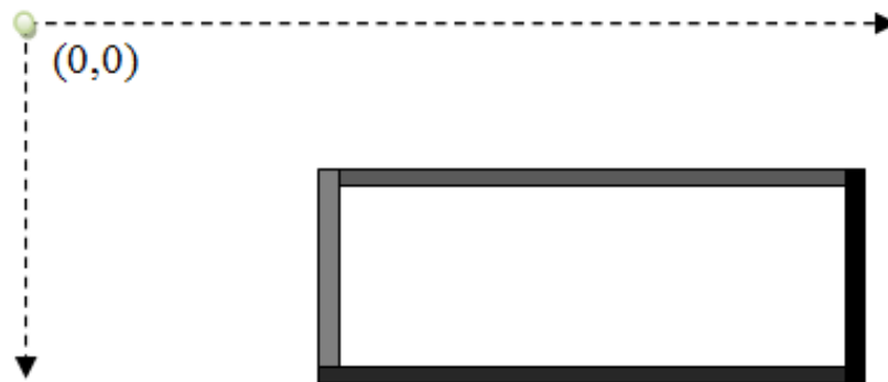
Figure 81: Wall Objects enclosing a space
