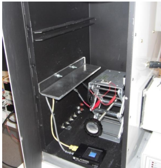
Fig. D: Picture of the inside of the dark housing showing a solar cell under test (lamp shutter closed). The reference cell is also shown although it is placed on the adjustable stage when reading light intensity.
