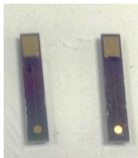
Figure 3.36: Comparison of colour changes observed at 1 mm gold disc electrode surface on an unmodified electrode (left) and on electrode after sol-gel electrodeposition (right).
