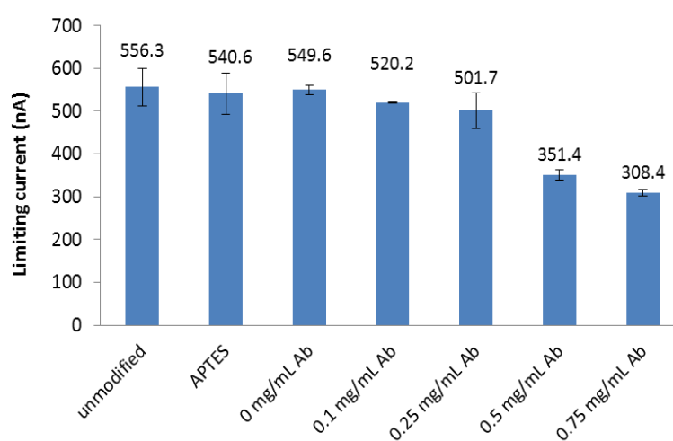
Figure 6.18: Reduction of limiting current calculated for the 10 \mu\text{m} microband array according to surface functionalization.
