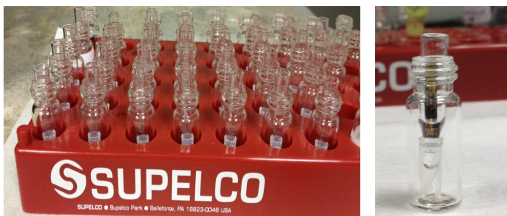
Figure 2.6 : Experimental set-up for surface biofunctionalisation using APTES silanisation methods for antibody immobilisation (left). A microinsert was used to accommodate the surface functionalisation on the working surface electrode (right).
