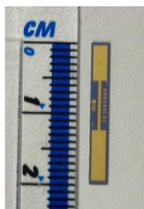
Figure 5.20: Picture of gold macroelectrode with 20 mm x 70 mm surface.
