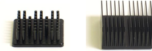
Figure 4.8: Heat sinks for MEMS and Bulk TEG Modules
