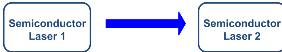
Figure 1.5: Basic diagram for optical injection-locking; if the light is injected unidirectionally from the Laser 1 to the Laser 2, the Laser 1 is known as master laser and the laser 2 is known as slave laser.
