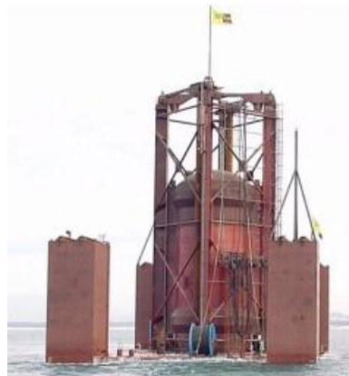
Figure 1.11: Original AWS prototype before submersion [31]
