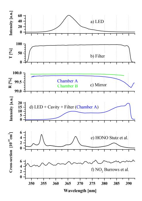
**Figure 2.** a) LED emission spectrum; b) filter transmission; c) Effective mirror reflectivity (smoothed) determined in chamber A and B experiments; d) empty cavity transmission spectrum (chamber A); e) HONO cross-sections by Stutz *et al.* (24); f) NO<sub>2</sub> cross-sections by Burrows *et al.* (25). Panels c) and d) refer to measurements with chamber A only.
