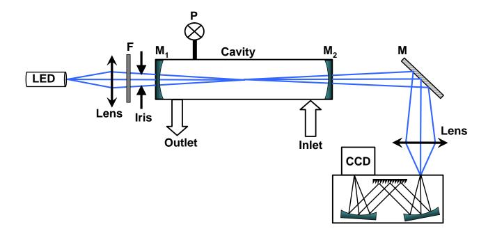
**Figure 1.** Schematic diagram of the experimental setup where LED is the light emitting diode, CCD is the charged coupled device, M is a metallic mirror,  $M_1$  and  $M_2$  are the high reflectivity dielectric mirrors centered at ca. 365 nm, F is a bandwidth filter, and P (chamber A) is a pressure gauge. The cavity length was 1.15 and 4.5 m for the two different gas chamber used in this study.
