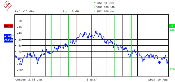
Fig. 2. Typical 802.15.4 distorted spectrum
