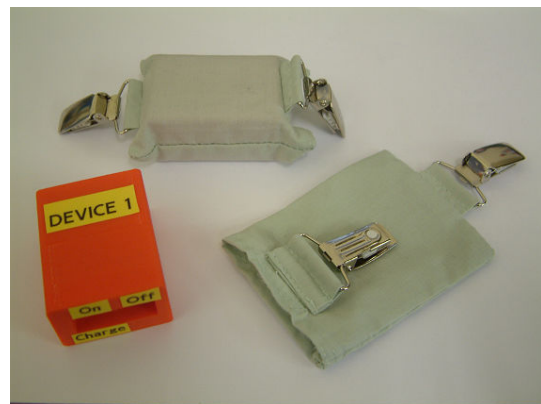
Figure 5. Cloth enclosure for WIMU ensuring the devices remain sterile while minimizing artifact introduction.
