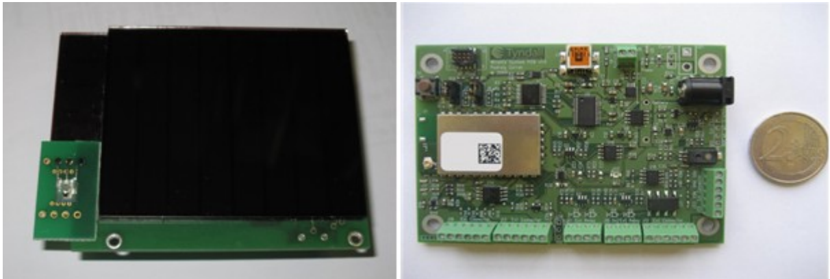
Figure 6. Implemented Indoor Light Powered WSN with Hybrid Energy Storage Compared to capacitive energy storage [1], the proposed hybrid energy storage solution reduces the average leakage current by 45% to 12.5 \mu A. The effective capacity of the energy storage is also increased 25% to 1.3 mAh.
