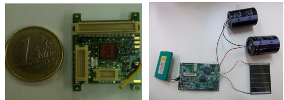
Fig. 2. Left: the GENESI v1.0 Main Layer prototype – with MSP430F5437 and CC2420 RF transceiver. Right: The Smart Power Unit prototype with solar EH, Li-ion rechargeable battery and supercapacitors.
