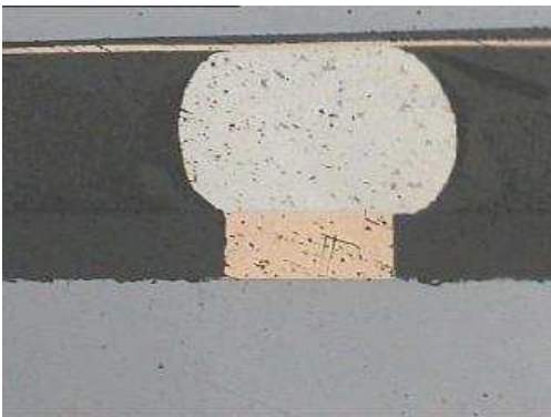
Figure 11 Solder ball attachment of pillar to inductor.
