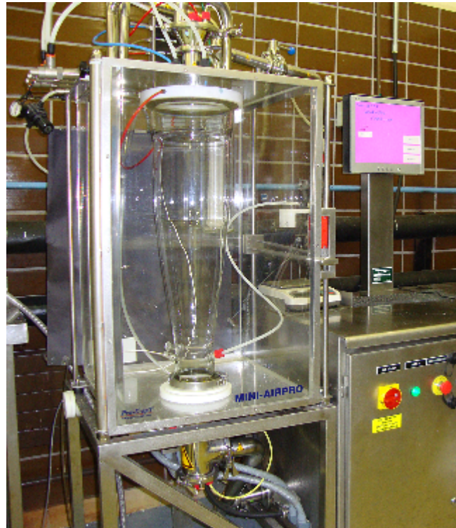
Figure 2.3: Laboratory scale of fluidised bed granulator employed in this study (Mini-Airpro, ProcepT, Belgium)
