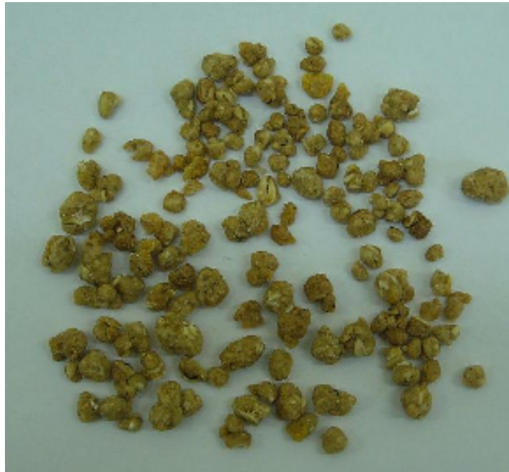
Figure 3.2: Granola produced by high shear granulation
