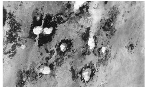
Figure 2. A Treated Specimen with Corrosion.
