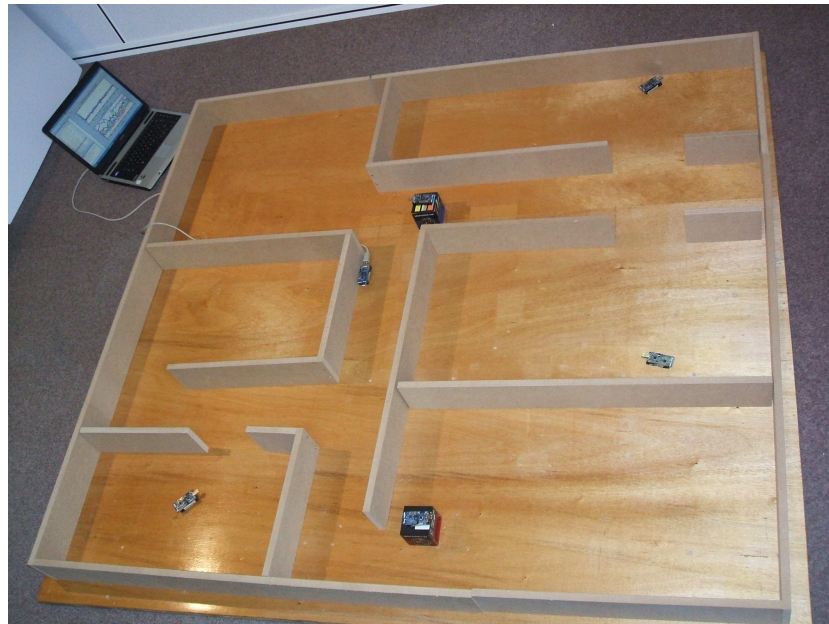
Figure 7. 802.15.4 Wireless experimental scenario.
