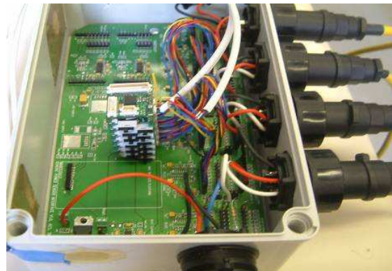
Figure 2: Multi-sensor interface board with sensors
