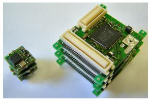
Fig. 3. 10mm and 25mm modular Tyndall nodes
