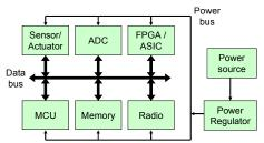
Fig. 1. Generic Wireless Sensor Node
