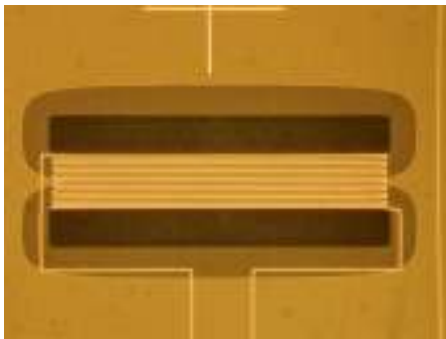
Figure 9: Microscope image of the active metal meander. The isotropic etch is visible.
