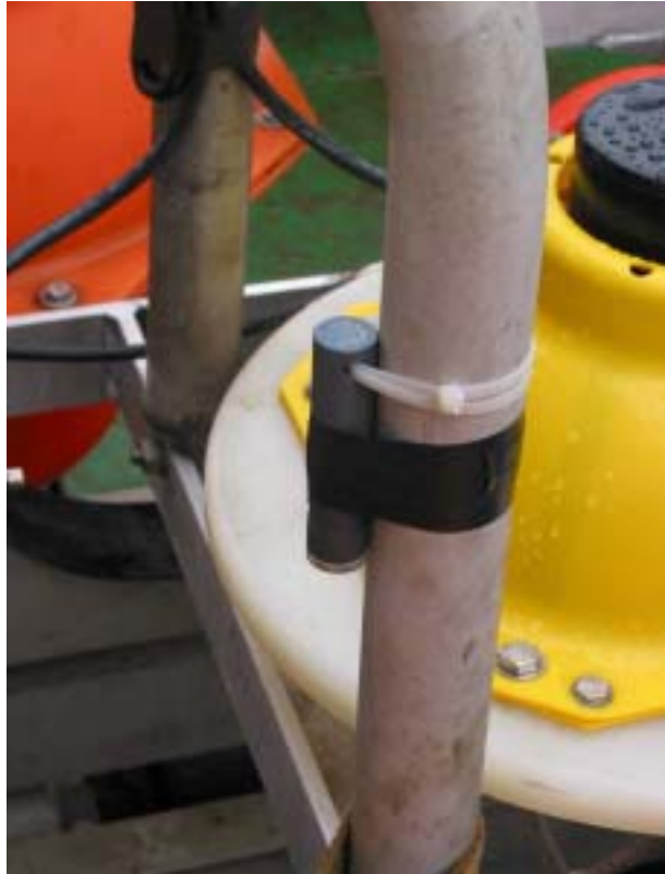
Figure 5.1e. Vemco minilog attached to ADCP frame
