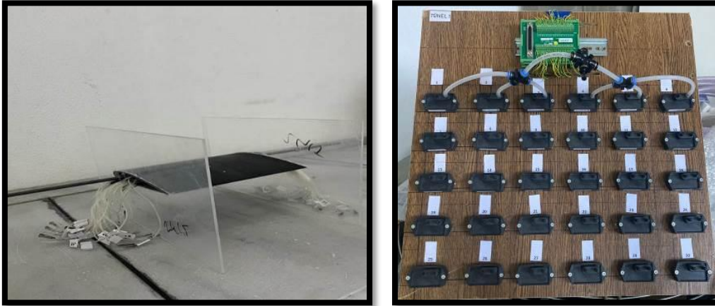
Figure 5. The sample of pressure test airfoil and diaphragm-type transducers.
