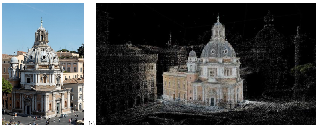
Figure 2: The church of Santa Maria di Loreto in Rome used to evaluate the fusion methodology. Real view (a), point cloud (b).
