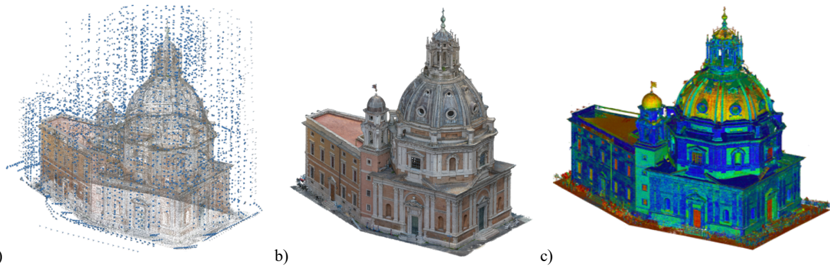
Figure 3: Data processing results: retrieved camera poses and sparse point cloud for some 4654 image (a) and colored dense point cloud (b) from Agisoft Metashape. The co-registered TLS point cloud (56 scans) shown with its intensity values (c).
