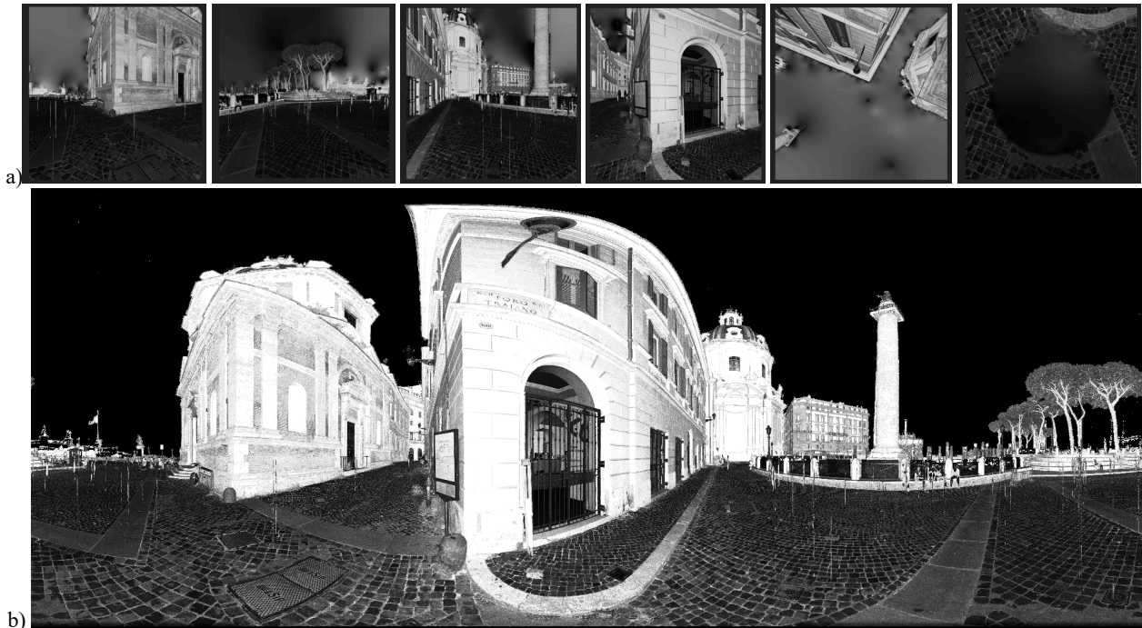
Figure 6: Examples of the TLS panoramic images - cubic (a) and equirectangular (b) - used to fuse scanning data and images.
