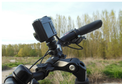
Fig. 3 -Adapter and one of the cameras attached to the handlebars of the bicycle.
