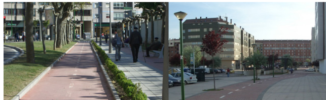
Figure 4 - Bicycle lane with and without segregation.
