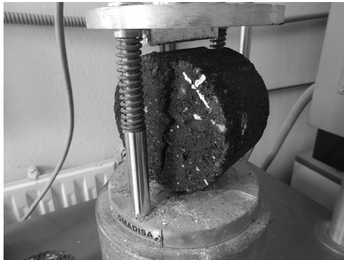
Fig. 2: Indirect tensile strength
