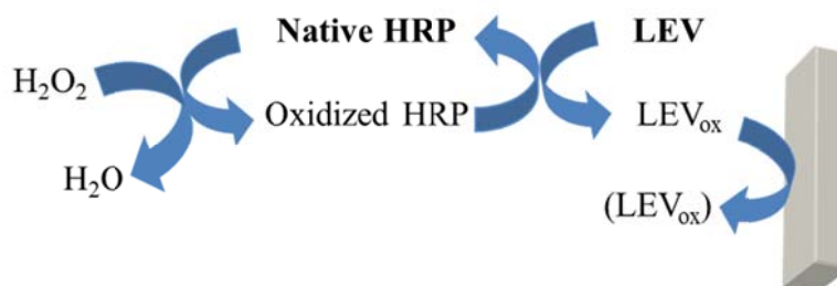
Figure 2.- Enzymatic mechanism for LEV determination
