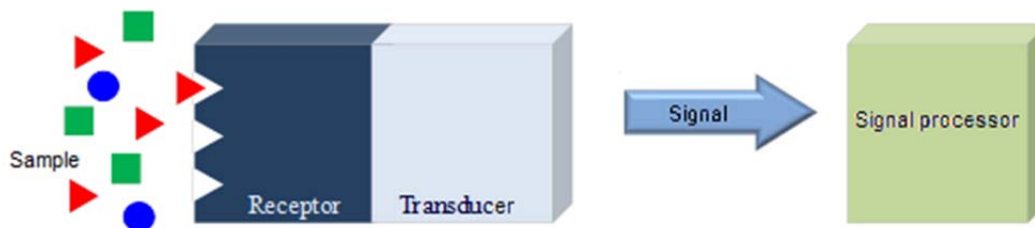
Figure 1 - Schematic diagram of the operation of a chemical sensor.
