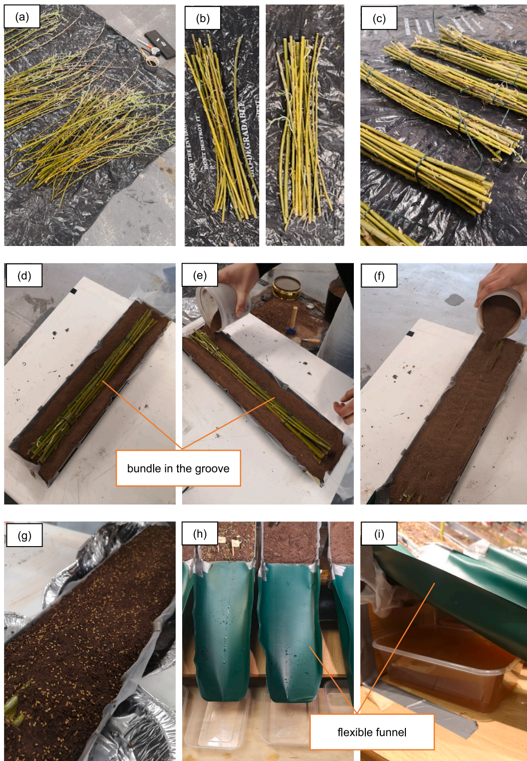
Fig. 3. Steps to build the LPD columns (Part 2). (a) Initial assembly of live cuttings and health assessment; (b) Live cuttings clipped and grouped together, striving a similar bundle diameter; (c) Tied bundles at 100 mm of each end; (d) Bundle placed in the groove made in the soil column; (e) Sides of the bundle being covered with soil; (f) Total bundle coverage; (g) Sown alfalfa seeds under the W + A treatment; (h) Flexible funnel installed above the soil at the toe of each column to allow surface runoff collection; (i) Container placed below the flexible funnel to allow water collection of subsurface flow.
