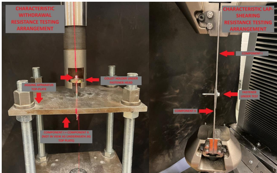
Figure 1 – Typical arrangements of characteristic withdrawal and lap-shearing resistance tests.
