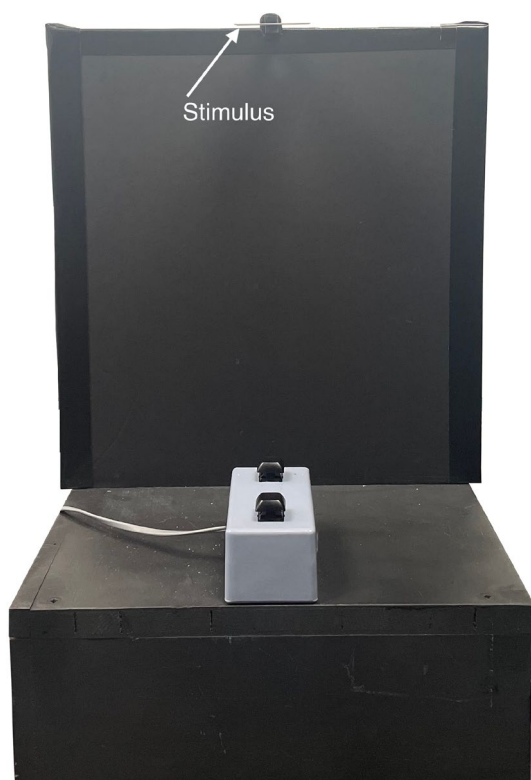
Fig. 2 Setup with example stimulus. At the beginning of each trial, the participants' index finger and thumb rested on the front button of the button box. After an auditory signal, they reached up to grasp the stimulus held in place by a clothes-peg. They placed the stimulus on the table and then placed their finger and thumb back on the front button
