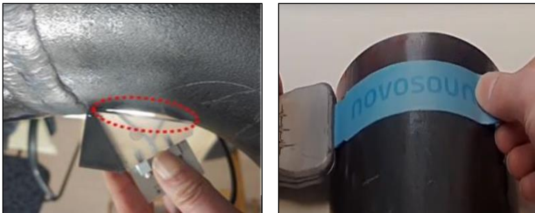
Figure 1: Problem in surface contact with a conventional rigid wedge transducer (left) [1]. Demonstration of the flexible Kelpie array inspecting a curved component (right).
