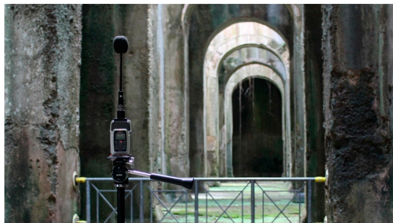
Figure 7. Equipment used during the acoustic survey within the piscina mirabilis .
