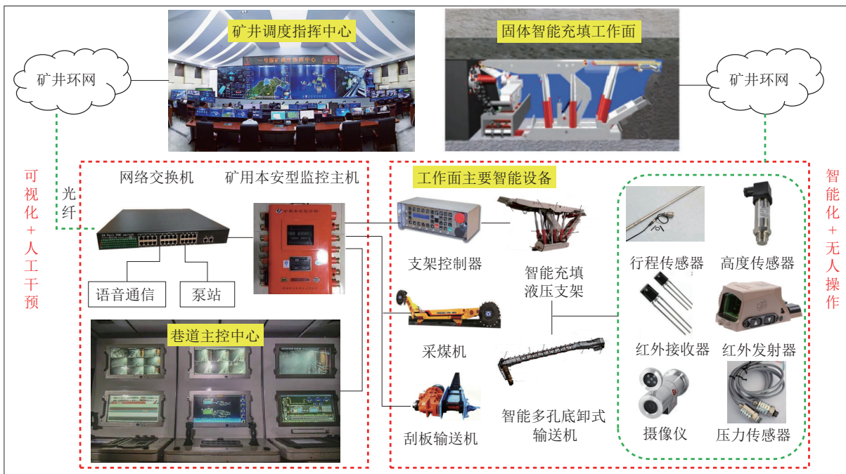
图 8 固体智能充填方法原理 [73] Fig.8 Principle of solid intelligent filling method [73]
