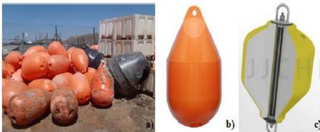
Figure 2.3 Different types of floating rafts used in Finisterra longlines system (Santos, 2013).
