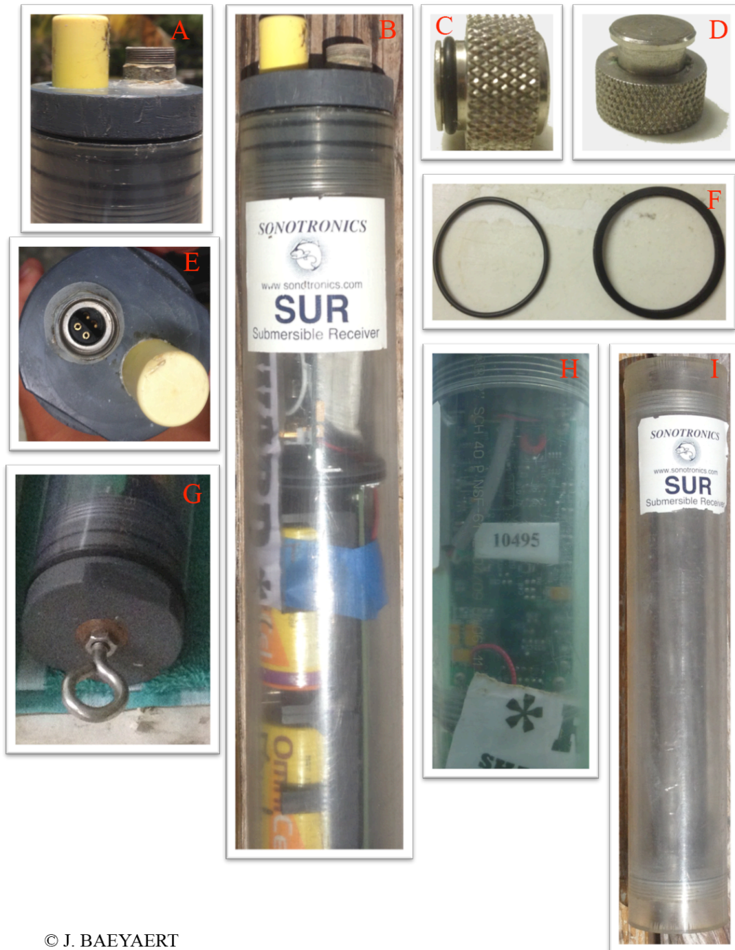
Fig. 2. Components and structure of a Submersible Ultrasonic Receiver “SUR” (Sonotronics Inc., ® Tucson, Arizona, U.S.A.). A: side view of the top lid of the SUR, revealing the transducer (yellow) and the serial connector bolt – the nut has been previously unscrewed -; B: mid-upper part of the SUR, exhibiting the two batteries; C & D: nut of the serial port connector; E: top view of the upper lid, showing the pin serial “COM” port connector; F: the two sorts of rubber gasket used to seal the SUR; G: Bottom of the SUR, showing the mounting eyebolt fixed to the lid; H: SUR serial number; I: empty SUR housing.
