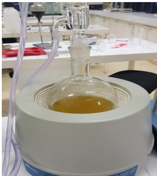
Fig.6: Photograph of reflux heating.
