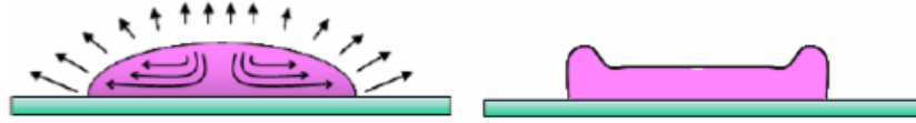
Fig. 2.5 - Illustration of the “coffee-ring” effect. Evaporation rate (represented by upward arrows) is highest at the edges of a printed droplet resulting in an accumulation of the solute at the periphery at the end of the drying process [8].
