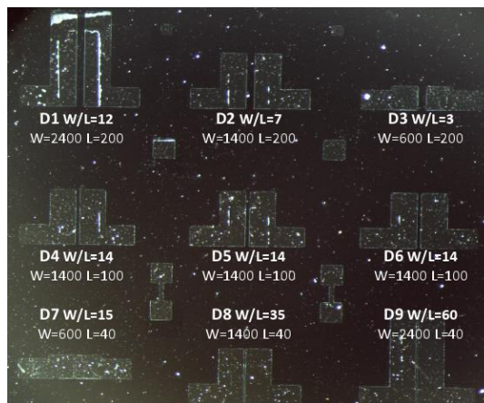
Fig. 4.2 - Photograph of a wafer of nine SiO 2 +ZTO transistors with each ratio per transistor. The dimensions W and L are in micrometers.
