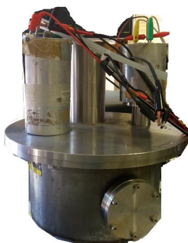
Figure 3.8 - Cryostat where the temperature dependent experiments were made.
