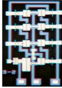
Figure 2.24 - Seven Stage RO based on ZnO TFT with 31 ns of propagation delay [70].
