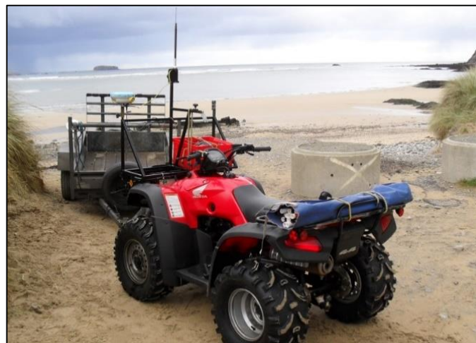
Figure 4.2: Field survey with DGPS' rover attached to a quad.
